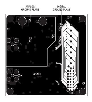
Figure 13. Bottom Side Showing Analog Ground Plane
