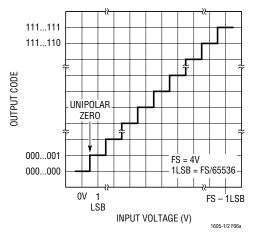
Figure 6a. LTC1605-1 Unipolar Transfer Characteristics
