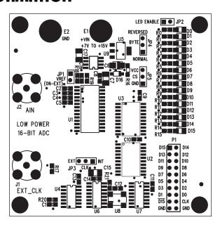
Figure 12. Component Side Silkscreen for the Suggested LTC1605-1/LTC1605-2 Evaluation Circuit
