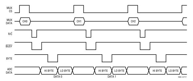
Figure 17. This Is the Timing Relationship Between the Selected MUX Channel, Its Conversion Data and the ADC and MUX Control Signals When Using the Sample Program In Listing 1. The Conversion Process Is Latency Free: the Data Is Always Generated Based On the Currently Selected MUX Input
