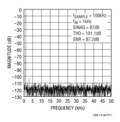
Figure 11. LTC1605-2 Nonaveraged 4096-Point FFT Plot
