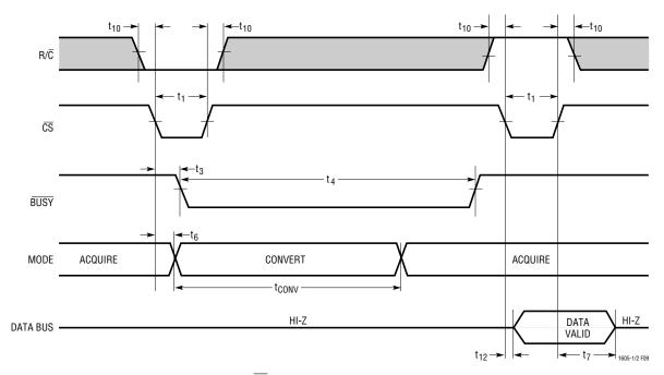
Figure 9. Using  $\overline{\text{CS}}$  to Control Conversion and Read Timing
