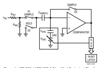
Figure 1. LTC1605-1/LTC1605-2 Simplified Equivalent Circuit
