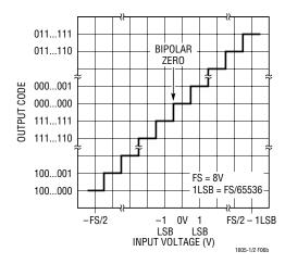
Figure 6B. LTC1605-2 Bipolar Transfer Characteristics
