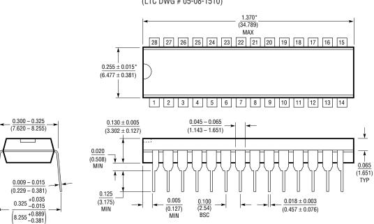
\*THESE DIMENSIONS DO NOT INCLUDE MOLD FLASH OR PROTRUSIONS. MOLD FLASH OR PROTRUSIONS SHALL NOT EXCEED 0.010 INCH (0.254mm)
