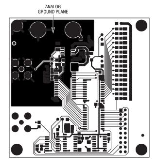
Figure 14. Component Side Showing Separate Analog and Digital Ground Plane
