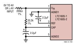
Figure 4. OV to 4V Input for the LTC1605-1 and ±4V for the LTC1605-2 Without Trim
