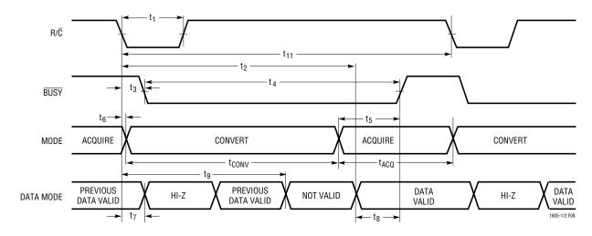
Figure 8. Conversion Timing with Outputs Enabled After Conversion (CS Tied Low)
