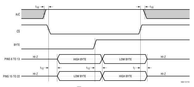
Figure 10. Using  $\overline{\text{CS}}$  and BYTE to Control Data Bus Read Timing
